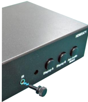
Front panel IR receiver -enabled
